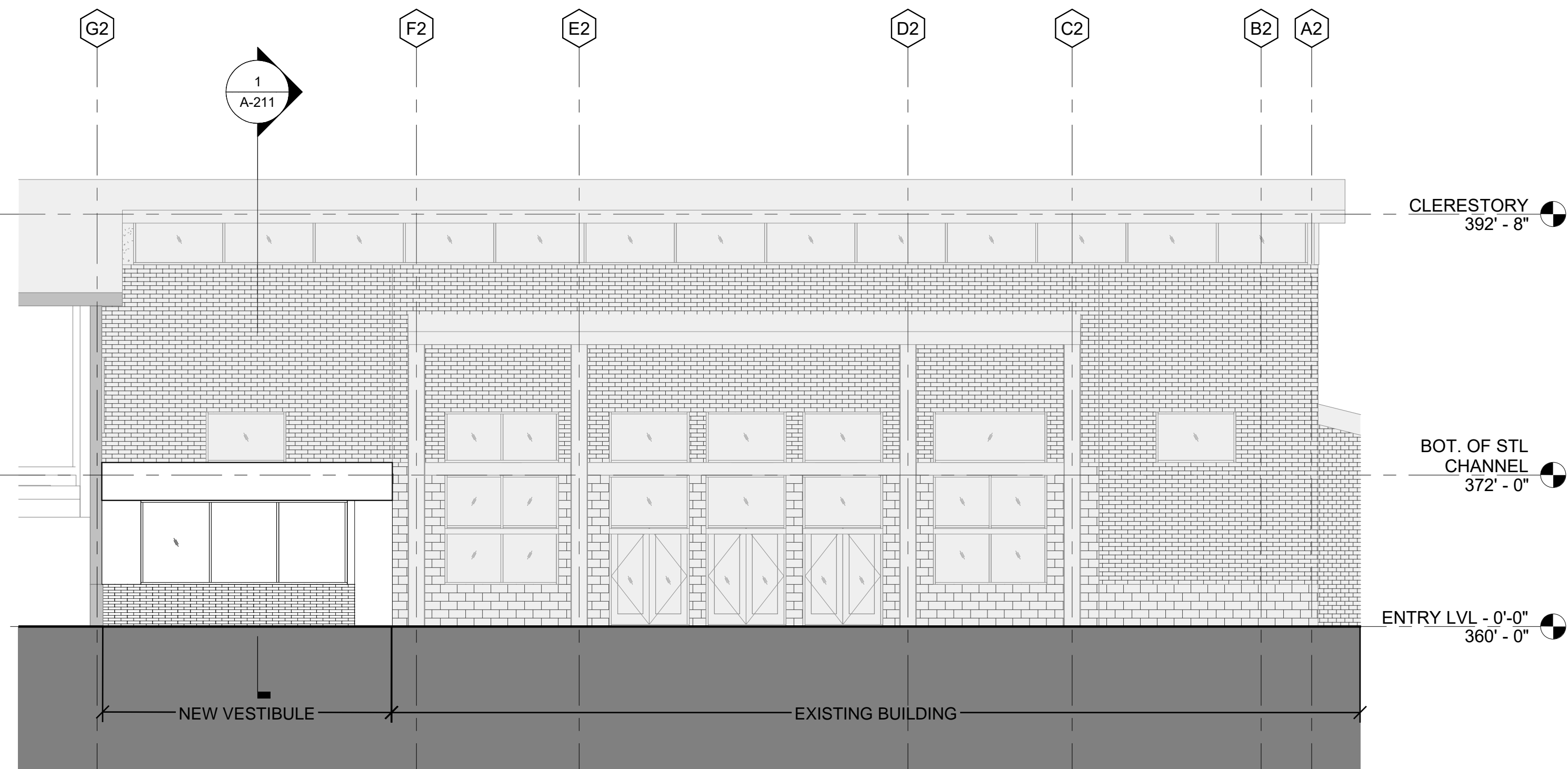
B1 EAST ELEVATION - ENTRY 1/8" = 1'-0"
