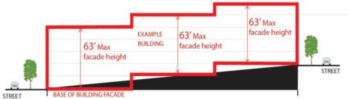
Figure 4 – Maximum Building Height
